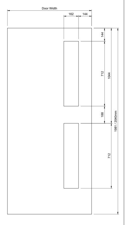
Description Doorpac Standard Aperture - 5G (DDA Compliant) - 150 x 700mm - 150mm Top & Side Margins & 150 x 700mm - 1050mm Top & 150mm Side Margins - FD60 Machining
